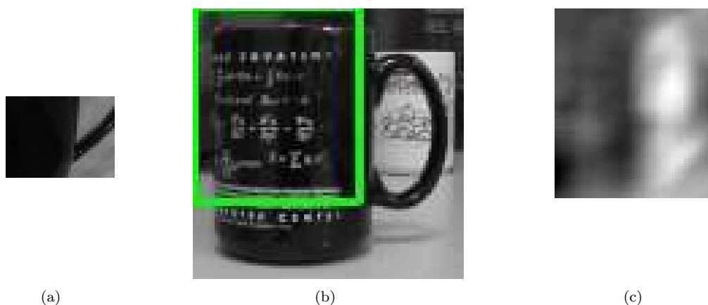
Figure 1: (a) A sample fragment, the one outlined in blue in the previous figure. (b) The new image we’re considering. We “slide” the fragment over this image and at each location we compute a similarity measure between the fragment and the image. The value at position (x, y) of the response corresponds to the similarity measure between the fragment and the image region that is overlapped when the fragment is placed with its upper lefthand corner at position (x, y) . Note that in order to keep the fragment within bounds its upper lefthand corner must stay within the region outlined in green. (c) The response image, which is exactly the size of the green region. White shows areas of high similarity.
