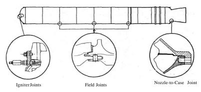
FIGURE 2. Locations and close-up views of booster-rocket field joints.
