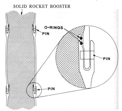
FIGURE 7. Joint rotation is caused by pressure from inside the rocket pushing the walls out farther than the joints. A gap opens, and hot gas flows past one or both of the 0-rings.
