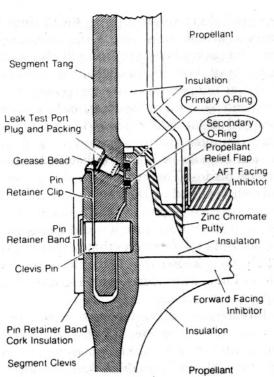
FIGURE 4. Detailed diagram of a field joint.
