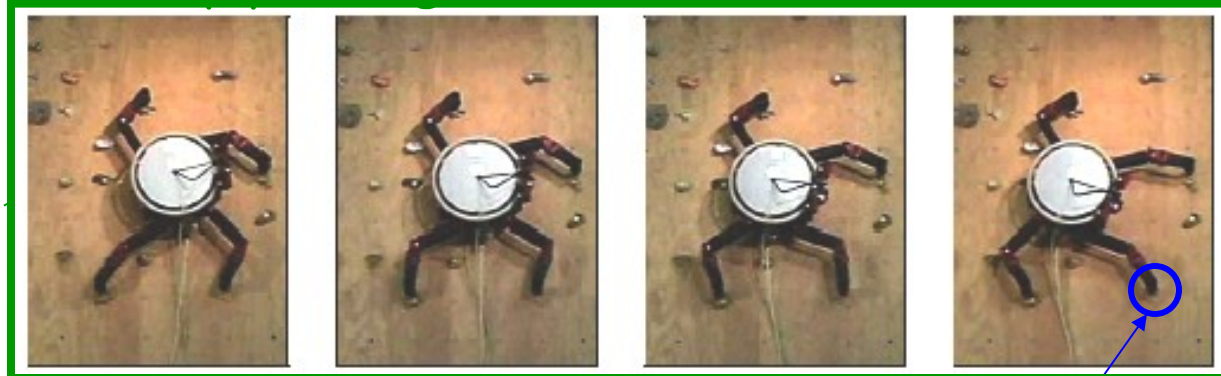
A one-step motion with a 4-hold stance, to remove the bottom right hand.
