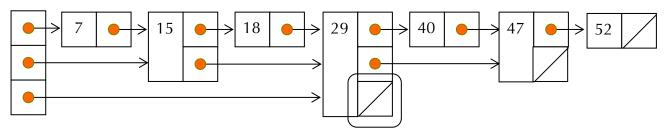
2.) Now we're on the 29 node and see that its level-2 pointer is **NULL**. There are lower levels to explore, so we stay on the same node, but descend from level 2 to level 1.
