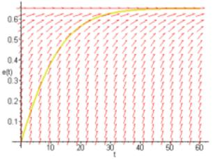
This approach does make a difference in both the rate of creep (faster) and the limiting strain (lower) compared to the case where E is independent of strain.
