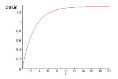
Two points are worth making. First, the limiting value dictated by the spring portion of the model is reached within a few seconds. Second, the strains predicted by our treatment are reality small, so the treatment with E = 3nRT is self consistent.
