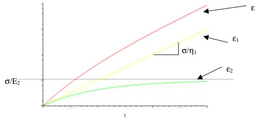
b) For this portion we want the strain for  $t>t_o$ . The stress is removed and the system allowed to relax. Again the strain is that for the two regions added. The dashpot at the top of the system cannot relax without a restoring force to cause it to contract. Since there is no such storing force (the applied stress is zero, not compressive), it remains strained to a value
