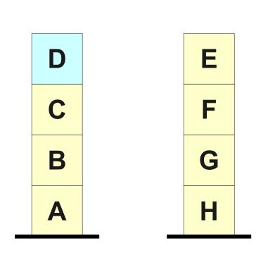
• Represent an infinite tape with two stacks.
