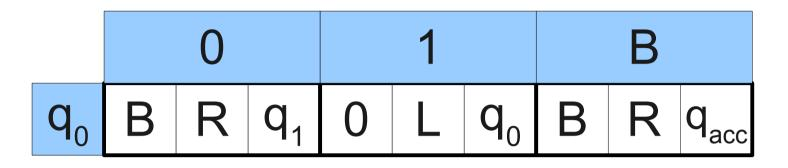
$// q_{0}$ 0: If reading 0, go to  $0q_0$ . 6: Write 0 1: If reading 1, go to  $1q_0$ . 7: Move left. 2: If reading B, go to  $Bq_0$ .
